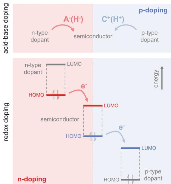
Fig. 9 Basic principle of acid–base doping, which involves the transfer of an anion ( $A^-$ , e.g.,  $H^-$ ) or cation ( $C^+$ , e.g.,  $H^+$ ) to the semiconductor (top); and redox doping, which involves the transfer of an electron to the LUMO or from the HOMO of the semiconductor in the case of n- and p-doping, respectively (bottom).
