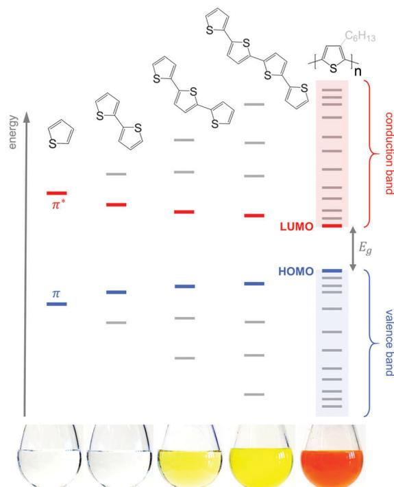
Fig. 3 Evolution of the HOMO and LUMO levels as well as bandgap  $E_g$  with increasing number of thiophene repeat units, resulting in valence and conduction bands for polythiophene; the images of 5 g L<sup>-1</sup> solutions in chloroform illustrate the narrowing of  $E_g$ , which leads to a red-shift in absorption (the polymer is P3HT). Note that crystallisation will lead to a further decrease in  $E_g$  due to electron delocalisation across adjacent chain segments.
