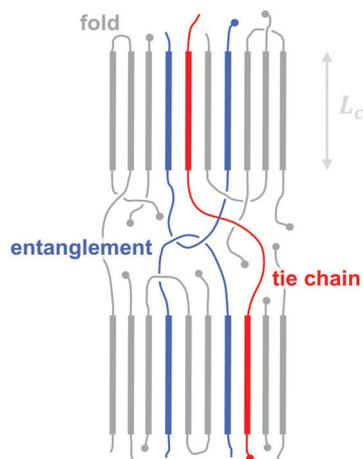
Fig. 7 Schematic nanostructure of a semi-crystalline polymer, indicating a chain fold that re-enters the same crystallite (with lamellar thickness  $L_c$ ), a tie chain that bridges two adjacent crystallites, and a chain entanglement that is trapped in the amorphous region between two crystallites.
