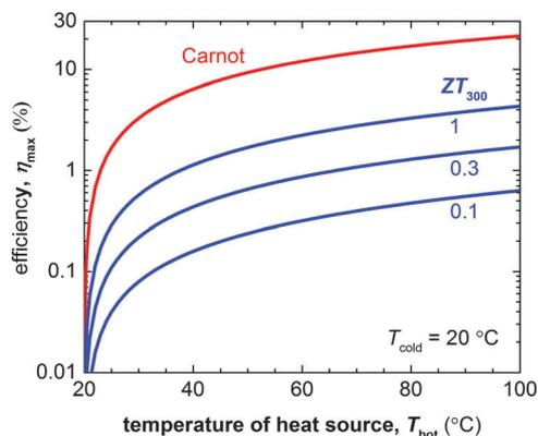
Fig. 15 The Carnot efficiency (red) and maximum efficiency  $\eta_{\max}$  of a thermoelectric leg (blue) with increasing heat source temperature  $T_{\text{hot}}$  (the heat sink is kept at  $T_{\text{cold}} = 20\text{ }^{\circ}\text{C}$ ). Eqn (8) was used to calculate  $\eta_{\max}$  for materials with a figure of merit at 300 K of  $ZT_{300} = 0.1, 0.5$  and 1.
