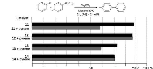
Fig. 3 Comparison of the catalytic activities of complexes **11–14** in the C–C Suzuki–Miyaura coupling of bromobenzene and *p*-tolylboronic acid. Grey bars indicate the activities in the presence of 10 mol% of pyrene.
