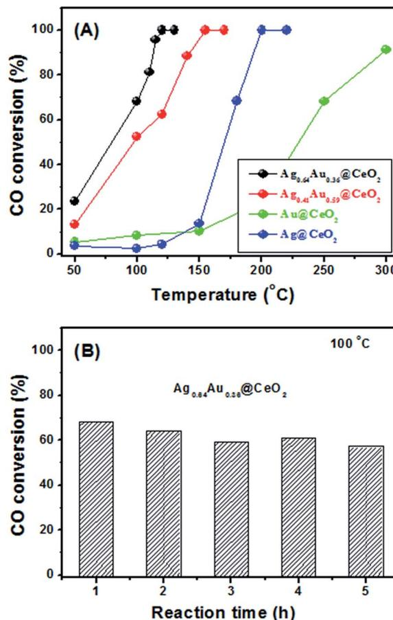
Fig. 4 (A) CO conversion curves of  $\text{Ag}@ \text{CeO}_2$ ,  $\text{Ag}_{0.64}\text{Au}_{0.36}@ \text{CeO}_2$ ,  $\text{Ag}_{0.41}\text{Au}_{0.59}@ \text{CeO}_2$  and  $\text{Au}@ \text{CeO}_2$ ; (B) cycling test of  $\text{Ag}_{0.64}\text{Au}_{0.36}@ \text{CeO}_2$  at  $100 \text{ }^\circ\text{C}$  for 5 h.
