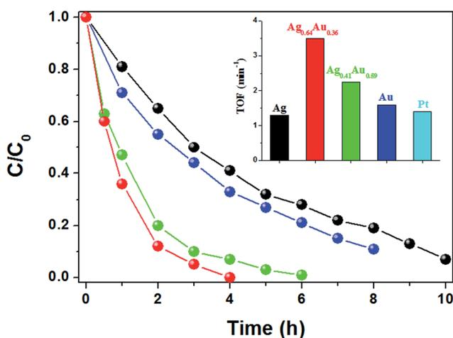
Fig. 3 Catalytic reduction of 4-NP by  $\text{Ag}@ \text{CeO}_2$  (black),  $\text{Ag}_{0.64}\text{Au}_{0.36}@ \text{CeO}_2$  (red),  $\text{Ag}_{0.41}\text{Au}_{0.59}@ \text{CeO}_2$  (green) and  $\text{Au}@ \text{CeO}_2$  (blue). Inset: calculated TOF compared with  $\text{Pt}@ \text{CeO}_2$ .<sup>7</sup>
