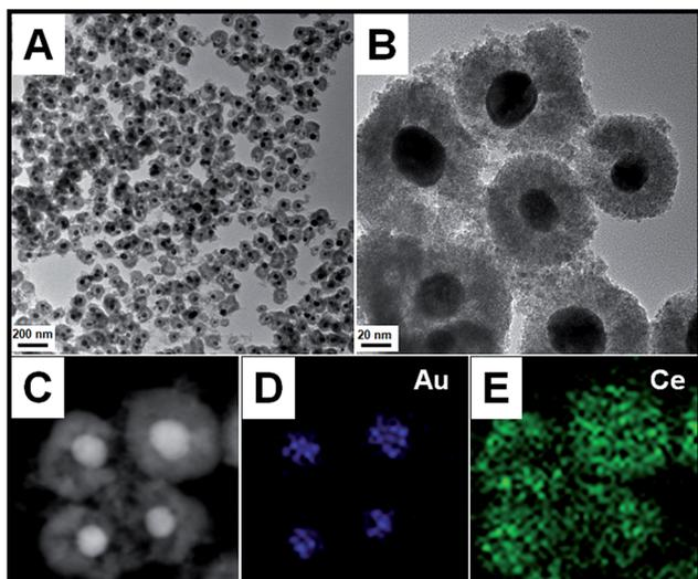
Fig. 2 TEM (A and B), and HAADF-STEM images (C to E) of Au@CeO<sub>2</sub>.
