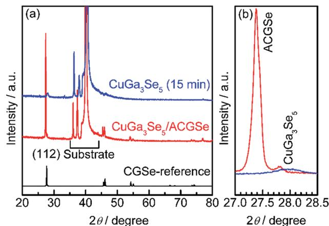
**Fig. 5** XRD patterns for CuGa<sub>3</sub>Se<sub>5</sub>/ACGSe with CuGa<sub>3</sub>Se<sub>5</sub> deposited for 15 min, and a reference CuGa<sub>3</sub>Se<sub>5</sub> film deposited on Mo/Ti/SLG for 15 min (a), and the corresponding (112) diffractions (b). The reference pattern for CGSe (PDF no. 31-456) is shown at the bottom for comparison.
