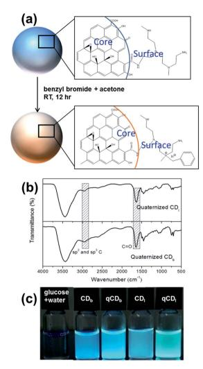
Fig. 5 (a) Illustration of the quaternization of PEI on the carbon dots. (b) FTIR spectra of the carbon dots quaternized with (a) branched PEI (CD<sub>b</sub>) and (b) linear PEI (CD<sub>l</sub>). (c) Optical images of (from L–R) glucose and water, CD<sub>b</sub>, quaternized CD<sub>b</sub>, CD<sub>l</sub>, quaternized CD<sub>l</sub> under UV lamp.
