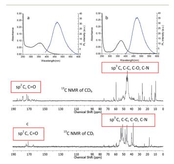
Fig. 3 UV-Vis absorbance and photo luminescent emission spectra (excited at 360 nm) of the carbon dots passivated with (a) branched PEI (CD<sub>b</sub>) and (b) linear PEI (CD<sub>b</sub>). (c) <sup>13</sup>C NMR spectrum of CD<sub>b</sub> and CD<sub>i</sub>.
