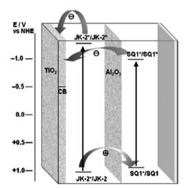
Fig. 9 Charge-transfer processes in multilayer co-sensitized TiO<sub>2</sub> films with a  $Al_2O_3$  layer (CB = conduction band, NHE = normal hydrogen electrode). Reproduced by permission of The Royal Society of Chemistry.
