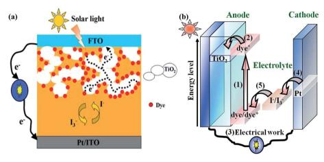
Fig. 1 (a) Schematic of a typical DSSC. (b) The basic sequence of events in a DSSC.
