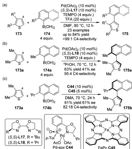
Scheme 50 The Pd-catalyzed synthesis of heterobiaryls reported by Yamaguchi and Itami.
