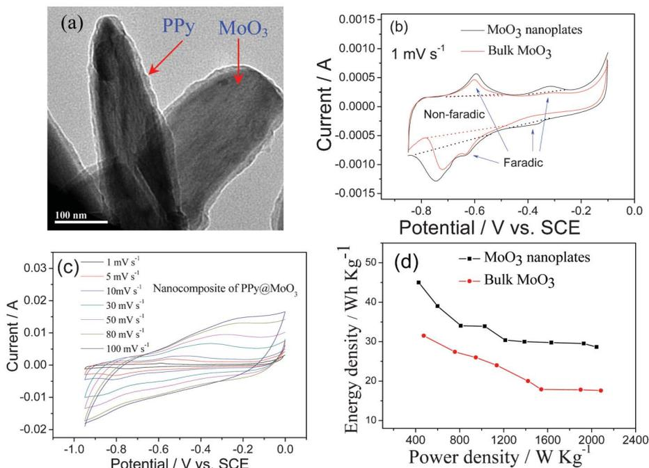
**Fig. 4** (a) TEM micrograph of PPY coated MoO<sub>3</sub> nanorods, (b) CV curves of the bulk and nanoplates MoO<sub>3</sub>, (c) CV curves of the PPY@MoO<sub>3</sub> nanocomposite at different scan rate and (d) Ragone plot of the ASCs based on MoO<sub>3</sub>//AC in 0.5 mol l<sup>-1</sup> Li<sub>2</sub>SO<sub>4</sub> solution (modified from ref. 6c and 49c).
