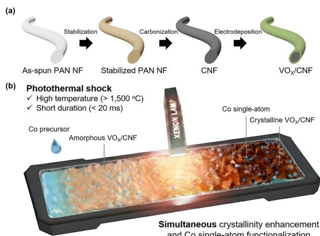
Fig. 1 (a) Schematic illustration of fabrication of amorphous VO x on CNF. (b) Schematic illustration of the synthesis of Co/VO x /CNF via ultrafast photothermal shock process, highlighting the simultaneous crystallinity enhancement and Co single-atom anchoring.
