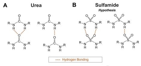
Fig. 1 Schematics of the (A) two potential H-bonding patterns in polyurea according to Mattia et al. 32 and (B) two hypothesized H-bonding patterns in polysulfamide.
