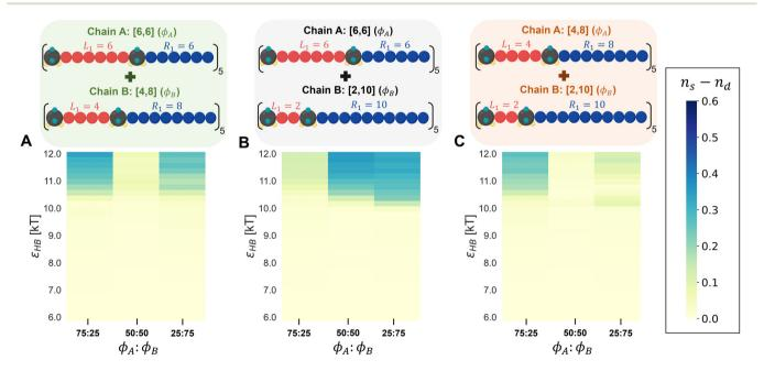
Fig. 9 Heat maps showing the difference in H-bonding between identical chain types  $(n_s)$  and different chain types  $(n_d)$  using the atomistically informed CG Config-1 model for the three mixtures - (A) [6,6] and [4,8], (B) [6,6] and [2,10], and (C) [4,8] and [2,10] - at varying H-bonding strengths (y-axis) and mixture compositions (x-axis).
