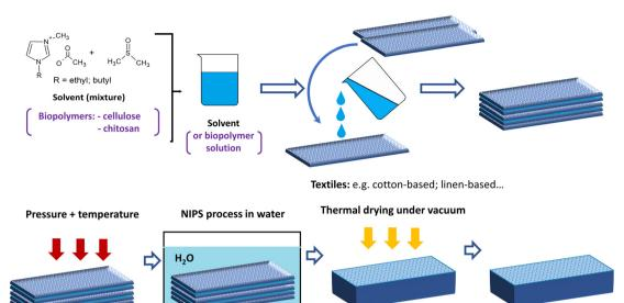
Fig. 1 Schematic description of the main fabrication steps used in the manufacture of the all biopolymer-based composites.
