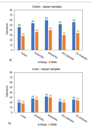
Fig. 6 Number of yarns per centimetre in the dry state for a) cottonbased and b) linen-containing composites.
