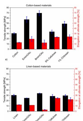
Fig. 10 Mechanical properties of precursor textiles and all-biopolymer composites a) cotton-based and b) linen-based (precursor materials were measured as a single layer).
