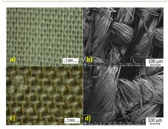
Fig. 2 The surface views by LM (a and c) and SEM (b and d) for the precursor textiles used in this work: (a and b) cotton cloth and (c and d) linen cloth.
