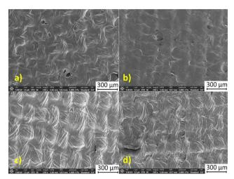
Fig. 3 The surface views (SEM) for the cotton-based composites prepared in this work: a) EmimOAc; b) BmimOAc; c) 8% cellulose and d) 1% chitosan
