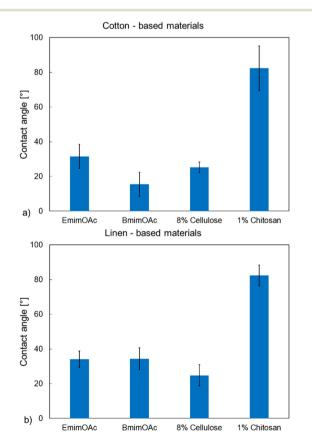
Fig. 7 The water contact angles for a) cotton-based and b) linencontaining composites.
