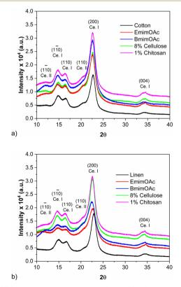
Fig. 8 XRD patterns for precursor textiles and laminar composites: a) cotton-based and b) linen-based.
