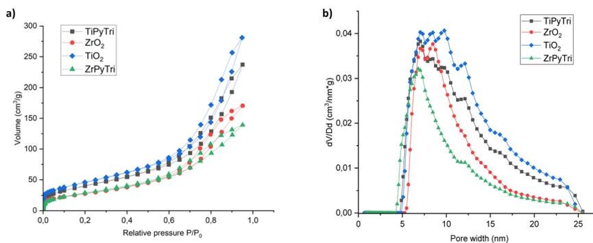
**Fig. 3** a) Nitrogen adsorption-desorption isotherms calculated using the DFT method for bare zirconia and titania, as well as for ZrPyTri2 and TiPyTri being demonstrative hybrids, and b) pore size distributions of the same materials.
