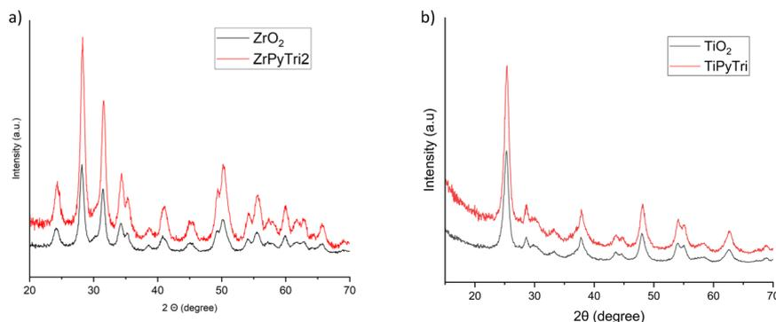
Fig. 5 Powder XRD patterns presented for a) bare zirconia and ZrPyTri2, and b) bare titania and TiPyTri.
