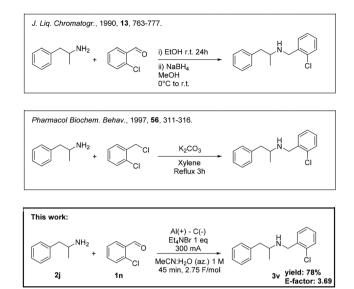
**Scheme 5** Clobenzorex synthetic approach and our approach *via* ERA. Reaction conditions: **1m** (3 mmol), **2j** (3 mmol), tetraethylammonium bromide (3 mmol), aluminium cathode and graphite cathode, MeCN : H<sub>2</sub>O (az.) (3 mL), 300 mA until a 2.75 F mol<sup>-1</sup> charge is passed (*ca.* 45 minutes). The product has been isolated as a hydrochloride salt.
