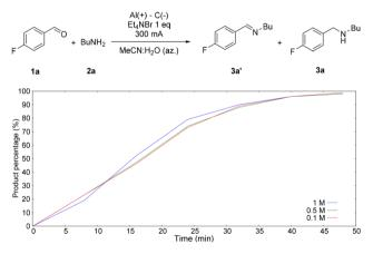
Fig. 2 Reaction kinetics. Reaction conditions: 1a (3 mmol), 2a (3 mmol), tetraethylammonium bromide (3 mmol), 300 mA. Blue line: 1 M: MeCN: H<sub>2</sub>O (az.) (3 mL), samples taken every 8 minutes for up to 48 minutes of reaction. Green line: 0.5 M: MeCN: H<sub>2</sub>O (az.) (6 mL), samples taken every 8 minutes for up to 48 minutes. Red line: 0.1 M: MeCN: H<sub>2</sub>O (az.) (30 mL), samples taken every 8 minutes for up to 48 minutes for up to 48 minutes.
