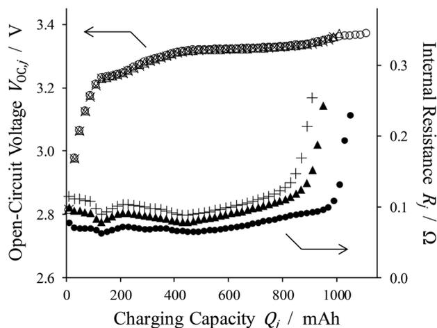
**Fig. 5** Reference data for cells N, D1, and D2. Open circle, open triangles, and crosses indicate the OCV of cells N, D1, and D2, respectively. Filled circles, filled triangles, and plus signs represent the internal resistance of cells N, D1, and D2, respectively.
