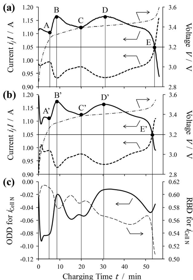
**Fig. 6** (a) Observed current distribution for cells N and D2 connected in parallel. (b) Calculated current distribution using reference data from cells N and D2. In both panels, the solid line represents the charging current flowing into cell N, the dashed line represents the charging current flowing into cell D2, and the dash-dotted line represents the module voltage. (c) Calculated ODD (solid line) and RBD (dashed line) values for cell N obtained during the analysis.
