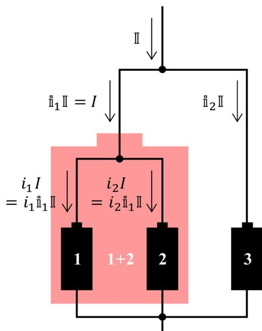
**Fig. 3** An example illustrating how cells are grouped and currents are calculated. First, the total current  $I$  is split between the composite cell (cells 1 + 2) and cell 3 in a two-cell distribution simulation. During that simulation, the current allocated to the composite cell (cells 1 + 2) is further split between cell 1 and cell 2 in a second two-cell distribution simulation.
