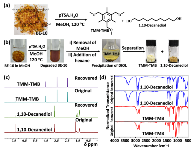
Fig. 3 (a) Scheme of BE-10 degradation using methanol. (b) Pictorial representation of the degradation of BE-10 and the recovery of the monomers, (c) 1 H NMR and (d) FT-IR comparison of the original and recovered monomers.
