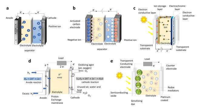
Fig. 20 Typical structures of the four most common applications of polymer electrolytes. Schematic of (a) a battery; (b) a double-layer capacitor; (c) an eletrochromic devices, (d) a hydrogen fuel cell; and (e) a dye-sensitized solar cell
