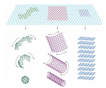
Fig. 17 Graphene as the building block for other carbon allotropes. It can be wrapped up to form fullerenes (in green), rolled up into carbon nanotubes (in violet), or stacked up to form graphite (in blue). It can be wrapped up into 0D buckyballs, rolled into 1D nanotubes, or stacked into 3D graphite. Reproduced from ref. 393 with permission from Springer Nature, copyright © 2007.
