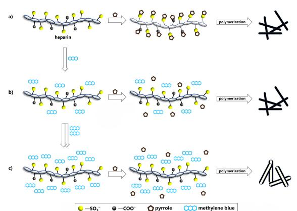
Fig. 14 (a). Simplified schematic representation of the possible mechanism for the formation of nanowires from the reaction of HEP with PPy. (b) and (c) Effect of the introduction of methylene blue into the system: (b) a small amount of methylene blue will still lead to the formation of nanowires, while (c) a higher methylene blue content will lead to the generation of PPy nanotubes.
