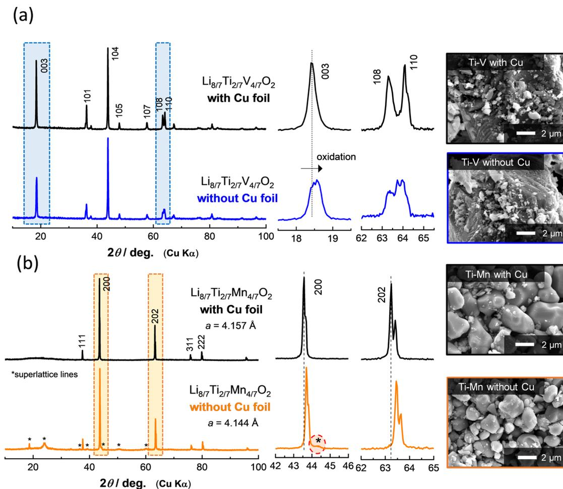
Fig. 2 XRD patterns and SEM images of (a)  $\text{Li}_{8/7}\text{Ti}_{2/7}\text{V}_{4/7}\text{O}_2$  and (b)  $\text{Li}_{8/7}\text{Ti}_{2/7}\text{Mn}_{4/7}\text{O}_2$  synthesized with or without Cu foil.
