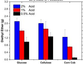
Fig. 6 Ethyl levulinate (g) and diethyl ether (g) produced from the sulphuric acid-catalysed ethanolysis of glucose, cellulose, and corn cob (5, 10, and 20 mass %) for three different feedstock-to-acid ratios (10:1, 20:1, and 40:1) for a reaction time of 6000 minutes at 150 °C.
