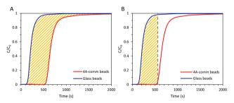
Fig. 2 (A) Area between the breakthrough curve of the glass beads and that of the adsorbent (yellow) for CO2 adsorption capacity at full utilization; (B) area between the vertical line from the breakthrough time,  $t_{\rm h}$ , and the breakthrough curve of the glass beads (yellow) for CO2 adsorption capacity at breakthrough.
