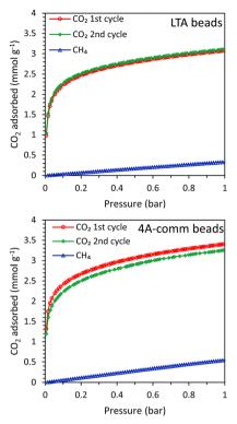
Fig. 3 CO<sub>2</sub> (2 cycles) and CH<sub>4</sub> adsorption isotherms of the LTA beads (top) and 4A-comm beads (bottom)
