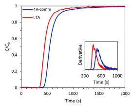
Fig. 4 CO<sub>2</sub> breakthrough curves of the LTA and 4A-comm beads. In the inset, the derivative of the breakthrough curves is displayed. Feed: 40 vol% CO<sub>2</sub> and 60 vol% CH<sub>4</sub> (mimicking biogas)
