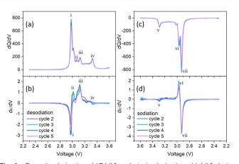
Fig. 4 Capacity derivatives (dQ/dV) and strain derivatives ( $d\epsilon/dV$ ) during (a) and (c) desodiation and (b) and (d) sodiation process, respectively during galvanostatic cycling.
