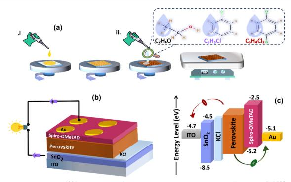
Fig. 1 The schematic representation of (a) fabrication process of solution-processed planar heterojunction perovskite solar cells PHJ PSCs by applying different anti-solvents (EtOH, CB, and DCB). (b) The final device architecture of PHJ PSCs. (c) Energy bands alignment between electrodes, charge transport layers, and halide perovskites facilitate efficient electron injection into SnO<sub>2</sub>/KCl and hole injection into spiro-OMeTAD layers.
