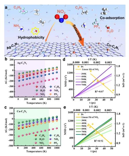
Fig. 6 (a) Schematic diagram of the high selectivity and hydrophobicity of  $Cu/Ag-C_2N_1$ . The Gibbs free energy of the six gases on (b)  $Ag-C_2N_1$  and (c)  $Cu-C_2N_1$  as a function of temperature. Gas diffusion and mean-squared displacement on (d)  $Ag-C_2N_1$  and (e)  $Cu-C_2N_1$  at different temperatures.
