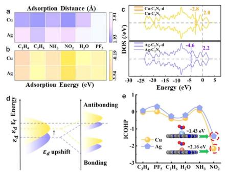
Fig. 4 (a) The adsorption distance and (b) adsorption energy of gases  $(C_2H_4, C_2H_6, NH_3, NO_2, H_2O, and PF_5)$  on the  $Ag-C_2N_1$  and  $Cu-C_2N_1$  monolayers. (c) The d-band center of  $C_2N_1$  doped with metals (Cu and Ag). (d) Metal-adsorbate interaction by altering the metal d-band center. (e) ICOHP of gases on the  $Ag-C_2N_1$  and  $Cu-C_2N_1$  monolayers.
