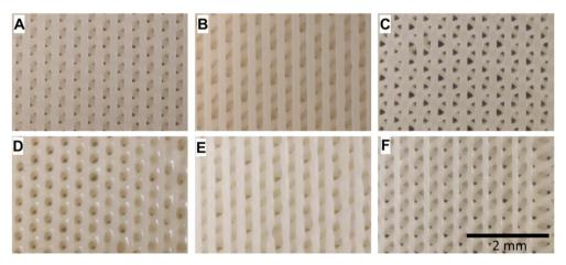
Fig. 19 Digital images showing nanocomposite scaffolds in their original printed state. (A–C) Underside (base) and (D–F) upper surfaces of the scaffolds (reproduced from ref. 150 with permission from Elsevier, Copyright 2021)
