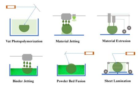
Methods used in biopolymer additive manufacturing (reproduced from ref. 14 with permission from Elsevier, Copyright 2023).
