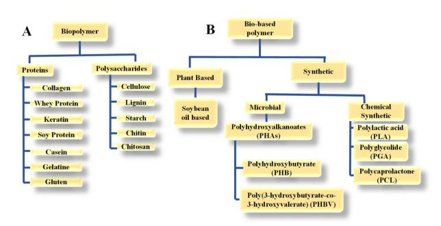
Fig. 2 Classification of (A) biopolymers and (B) bio-based polymers.
