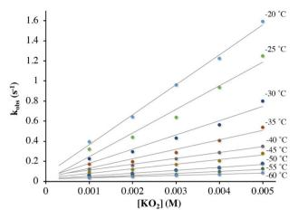
Fig. 6 Temperature-dependent rate constants,  $k_{\rm obs}$ , for the formation of superoxo 2 in the reaction between 3 and KO<sub>2</sub> (solubilized with KryptoFix) in THF, plotted against [KO<sub>2</sub>]. The  $\sim$  zero intercepts would be consistent with irreversible O<sub>2</sub>. binding. [Fe(III)] = 0.1 mM. Concentrations listed correspond to after mixing in the stopped-flow cell
