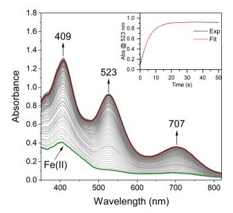
Fig. 1 Time-resolved spectral changes obtained upon mixing THF solutions of five – coordinate [Fe<sup>II</sup>(S<sub>2</sub><sup>Me2</sup>N<sub>3</sub>(Pr,Pr))] (1, 0.25 mM) and O<sub>2</sub> (3.95 mM) at -40 °C. Inset: kinetic trace ( $\lambda=523$  nm) showing the formation of the Fe–O<sub>2</sub> intermediate 2. All reported concentrations are after mixing in the stopped-flow cell.
