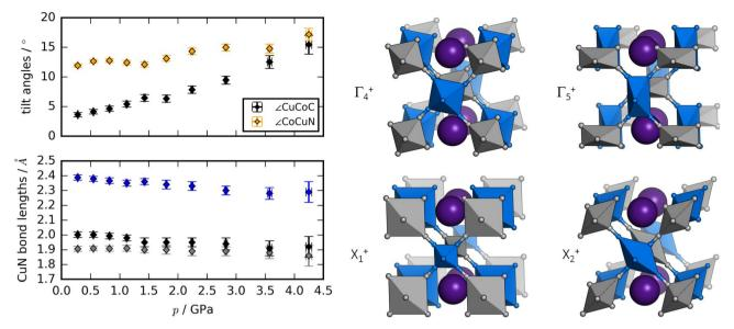
Fig. 3 The left panel shows the pressure evolution of the tilt angles of RbCuCo, with ∠CuCoC in black and ∠CoCuN in orange, and the CuN bond lengths of RbCuCo as a function of pressure. The right panel visualises the distortion modes (with exaggerated amplitudes) potentially driving the phase transition in RbCuCo.
