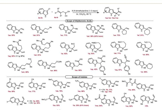
Scheme 2 Scope of allylboronic acids and indoles<sup>a</sup>. <sup>a</sup>Reaction conditions: 3-Cl-indole 2 (0.2 mmol, 1.0 equiv), allylboronic acid 4 (0.4 mmol, 2.0 equiv), N,N-dimethylaniline (0.2 mmol, 1.0 equiv), CH<sub>2</sub>Cl<sub>2</sub> (2 mL), 80 °C, under Ar; isolated yield.
