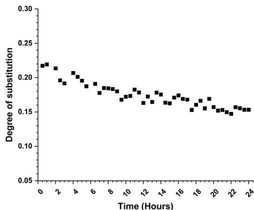
Fig. 2 Plot of degree of substitution from NMR experiment for cellulose *N*-phenylcarbamate reacting with EtOH at 80 °C. The DS values were determined from the diffusion edited  $^1\text{H}$  NMR with standard calibration curve.
