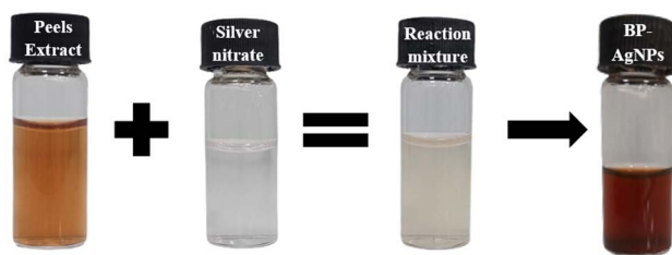
Fig. 5 Pictorial representation of BP-AgNPs synthesis. Extract combined with silver nitrate in a 1 : 10 ratio shows a pale color, which turned dark brown after incubation.
