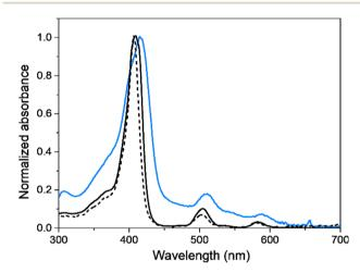
Fig. 4 Absorption spectra of  $\mathsf{TPPF}_{20}$  (black dashed line),  $\mathsf{EDOT}\text{-}\mathsf{TPPF}_{16}$  monomer (black continuous line) in ACN and  $\mathsf{PEDOT}\text{-}\mathsf{TPPF}_{16}$  electrodeposited polymer on ITO (cyan continuous line).
