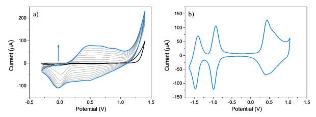
Fig. 3 (a) First (black), 2nd–9th (grey) and 10th (cyan) cyclic voltammograms of EDOT-TPPF<sub>16</sub>. The measurements were done in DCE containing TBAPF<sub>6</sub> (0.1 M) using an ITO working electrode. (b) Electrochemical response of the electropolymerized film PEDOT-TPPF<sub>16</sub> in ACN containing only TBAP (0.1 M). Scan rate:  $0.100 \text{ V s}^{-1}$ .
