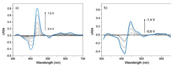
Fig. 5 Difference absorption spectra, ΔAbs, of: PEDOT-TPPF<sub>16</sub> film deposited over ITO electrode obtained at different applied potentials: (a) 0.4 (black line), 0.9 to 1.4 (gray lines) and 1.5 V (cyan line); (b) -0.8 (black line), -0.9 to -1.3 (gray lines) and -1.4 V (cyan line). All measurements were conducted in ACN (0.10 M TBAP) at 20 mV s<sup>-1</sup>
