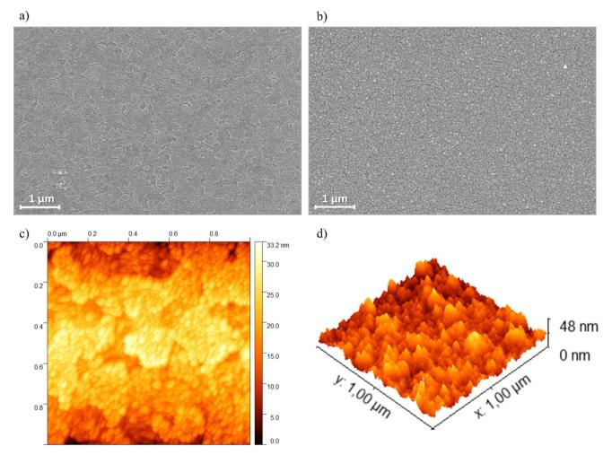
Fig. 6 SEM images of (a) bare ITO and (b) PEDOT-TPPF $_{16}$  film. Scale bars are 1  $\mu$ m. (c) AFM images of ITO electrode surface (scan size 1  $\times$  1  $\mu$ m) registered after electrodeposition of porphyrin film. (d) Three-dimensional representation of the electrode surfaces measured by AFM. Films were grown cycling in the same conditions of the exhibited in Fig. 3.
