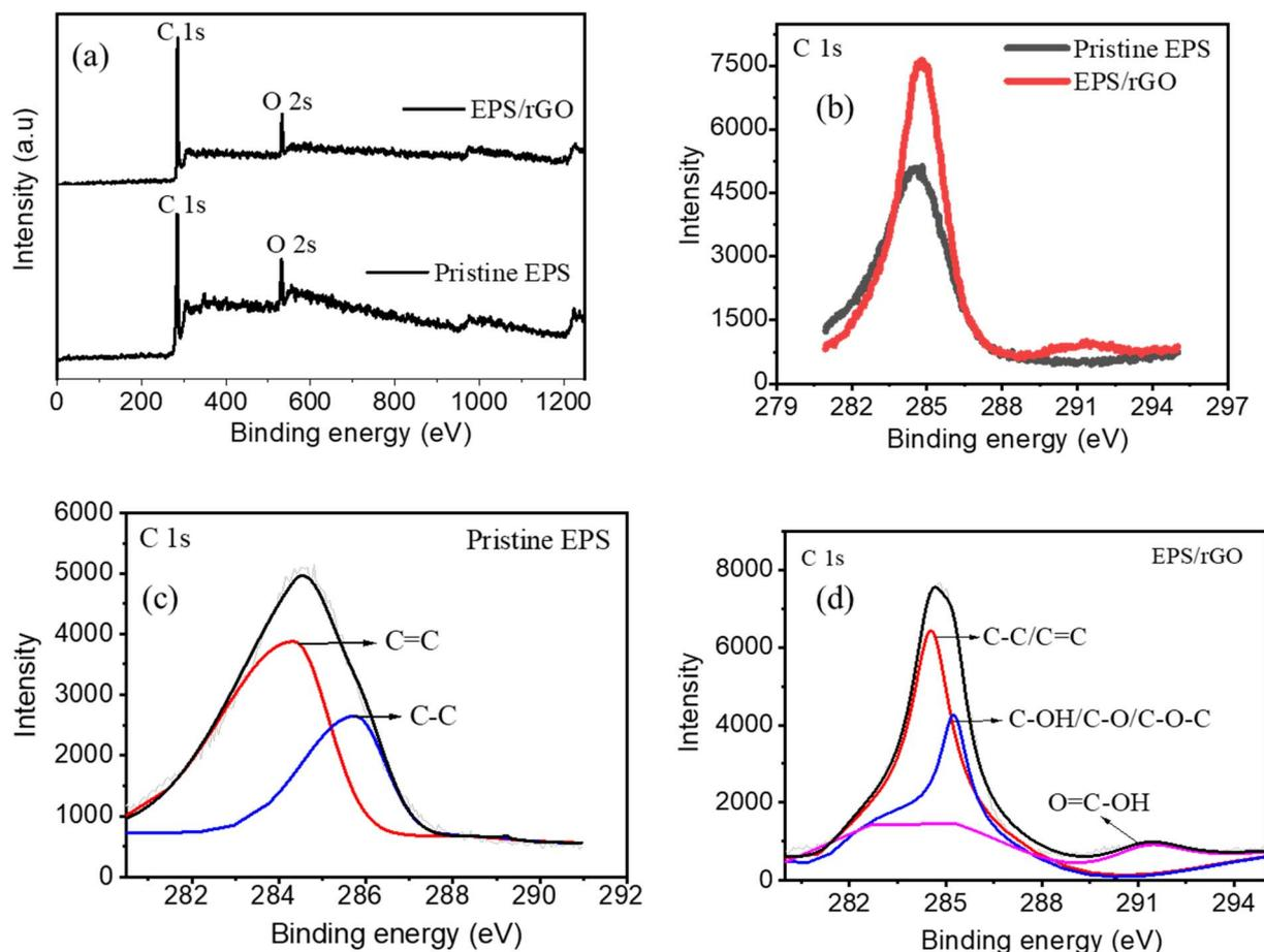
Fig. 4 (a) XPS spectra of pristine EPS and EPS/rGO composite (b) comparison of C 1s spectrum of pristine EPS and EPS/rGO composite (c) C 1s spectrum of pristine EPS (d) C 1s spectrum of EPS/rGO composite.
