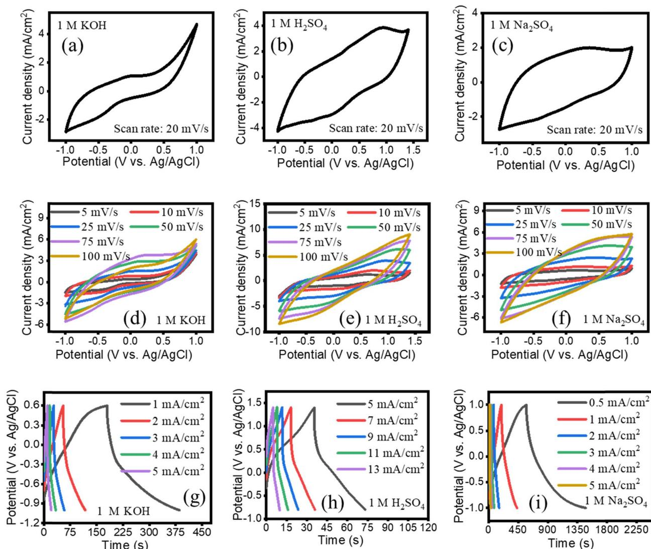
Fig. 5 (a, b, c) CVs at 20 mV s<sup>-1</sup> (d–f) CVs at various scan rates (g–i) GCD of EPS/rGO composite recorded in 1 M KOH, 1 M H<sub>2</sub>SO<sub>4</sub>, Na<sub>2</sub>SO<sub>4</sub> aqueous electrolyte.
