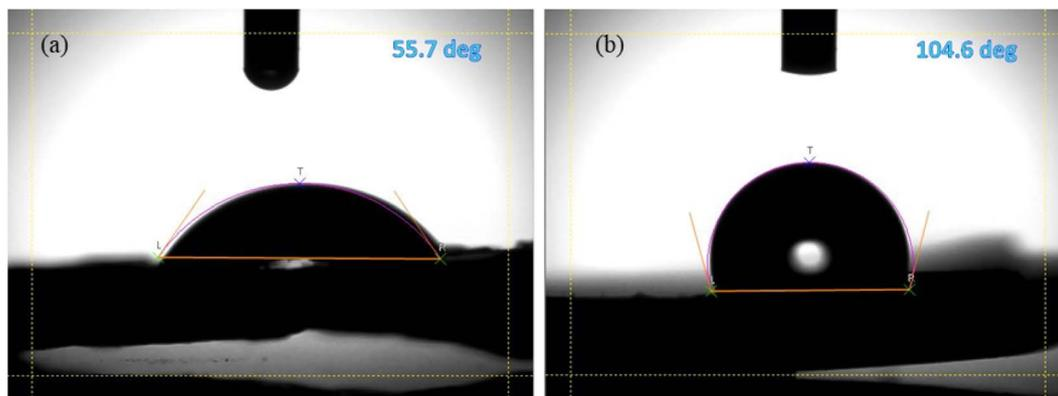
Fig. 3 The contact angles of (a) pristine EPS (b) EPS/rGO composite.
