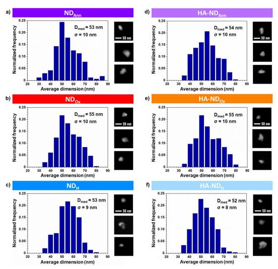
Fig. 2 Size distributions of the NDs derived from SEM images. Particle size histograms were constructed based on 300 NDs from 3–4 micrographs, except for ND<sub>Ann</sub>, where the distribution was derived from 168 NDs. Details from SEM micrographs showing ND particles are also presented. (a) ND<sub>Ann</sub>, (b) ND<sub>Ox</sub>, (c) ND<sub>H</sub>, (d) HA–ND<sub>Ann</sub>, (e) HA–ND<sub>Ox</sub>, and (f) HA–ND<sub>H</sub>.
