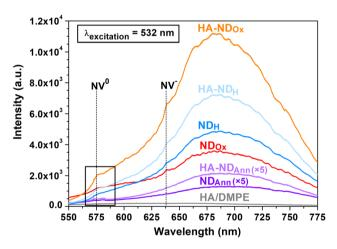
Fig. 4 Photoluminescence spectra of the NDs and the HA/DMPE conjugate. The PL spectra of ND<sub>Ann</sub> and HA-ND<sub>Ann</sub> are multiplied by a factor of five. The black rectangle identifies the region highlighted in Fig. 1b.
