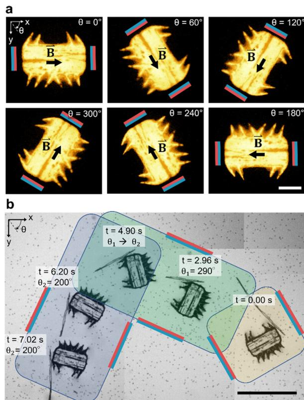
**Fig. 4** Magnetic manipulation of a soft polymeric microrobot. (a) Controlled rotational motion of a fluorescent microrobot in a glycerol/distilled water mixture (50/50 vol%). Scale bar, 100  $\mu\text{m}$ . In the stitched image sequence (b), the navigation of a microrobot along a 90-degree curved pathway using external magnetic field guidance and acoustic propulsion ( $f = 23.3 \text{ kHz}$ ,  $V_{\text{pp}} = 22.5 \text{ V}$ ) is shown. Scale bar, 500  $\mu\text{m}$ .
