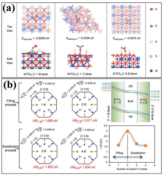
Fig. 13 (a) The adsorption energies of various SrTiO<sub>3</sub> crystalline facets to K<sub>2</sub>CO<sub>3</sub>; (b) work function values of {110} and {100} facets for K loaded SrTiO<sub>3</sub> at the work function variations, and conceptual band illustrations throughout the boundaries among the {110} and {100} facets of an exposed single K loaded SrTiO<sub>3</sub> catalyst. Adapted from ref. 306. Copyright © 2022, Elsevier.
