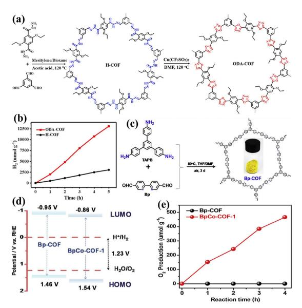
Fig. 19 (a and b) The process for the fabrication and photocatalytic HER of H-COF and ODA-COF. Adapted from ref. 400. Copyright © 2022, John Wiley & Sons, (c) Graphical depiction of the fabrication of Bp-COF, (d) the estimated HOMO/LUMO spectral positions and (e) the photocatalytic OER performance of Bp-COF and BpCo-COF-1. Adapted from ref. 401. Copyright © 2020, Elsevier.
