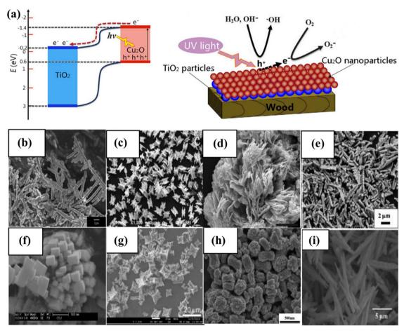
Fig. 6 (a) Depiction of the photocatalysis mechanism at the TiO<sub>2</sub>/Cu<sub>2</sub>O heterostructures, and a suggested model for the formation of negative oxygen ions on wood treated with TiO<sub>2</sub>/Cu<sub>2</sub>O under UV light. Adapted from ref. 116. Copyright © 2016, Springer Nature, (b-i) morphology of BiVO<sub>4</sub>.<sup>144</sup> This chapter is distributed under the terms of the Creative Commons Attribution 3.0 License.
