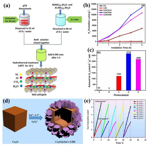
Fig. 20 (a-c) The fabrication procedure and photocatalytic HER of the NiAl LDH/g-C<sub>3</sub>N<sub>4</sub> nanocomposite. Adapted from ref. 409. Copyright © 2020, Elsevier, (d and e) graphical depiction of the synthesis and PWOS of Cu<sub>2</sub>O/ZnCr-LDH hollowed materials. Adapted from ref. 410. Copyright © 2017, Elsevier.
