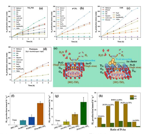
Fig. 11 (a-d) PWS using different photocatalysts having multiple sacrificial reagents.<sup>268</sup> (e-h) {001}- and {101}-faceted TiO<sub>2</sub> and PWS performance of Pt-Au/{001}-TiO<sub>2</sub> under light illumination. Adapted from ref. 279. Copyright © 2021, American Chemical Society.
