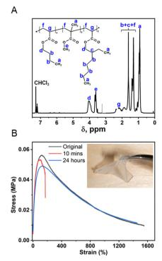
Fig. 3 (A) <sup>1</sup>H-NMR spectrum of the matrix polymer with characteristic chemical shift peaks marked on the chemical structure. (B) Tensile results of the cut matrix polymer that self-healed for 10 min and 24 h in comparison to the original uncut material.
