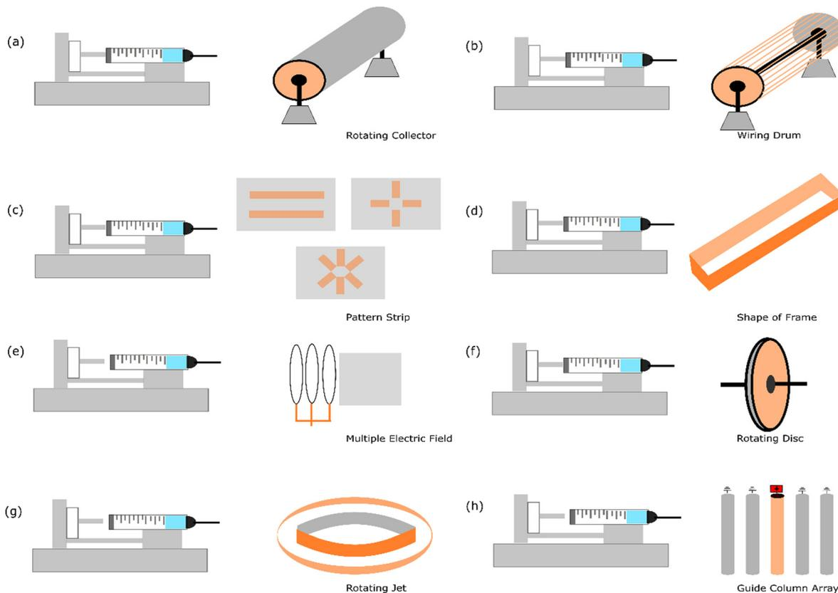
Fig. 3 Illustration of the current methods for aligning nanofibers using electrospinning: (a) increasing the speed of the rotating collector,<sup>14</sup> (b) wiring drum,<sup>58</sup> (c) patterned strip,<sup>57</sup> (d) shape of frame,<sup>59</sup> (e) multiple electric fields,<sup>10</sup> (f) rotating disc collector,<sup>9</sup> (g) rotating jet,<sup>60</sup> and (h) guide column array.<sup>13</sup>
