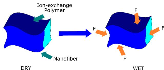
Fig. 8 Mechanism of the nanofiber suppressing the swelling of the matrix.<sup>92,93</sup>
