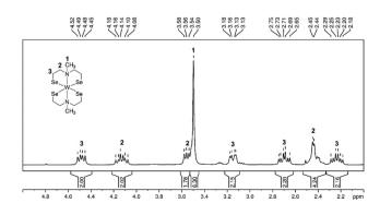
Fig. 1 <sup>1</sup>H NMR spectrum (CDCl<sub>3</sub>, rt) of complex [W{(SeC<sub>2</sub>H<sub>4</sub>)<sub>2</sub>NMe}<sub>2</sub>] with proton integration and assignment of protons to the molecular structure.
