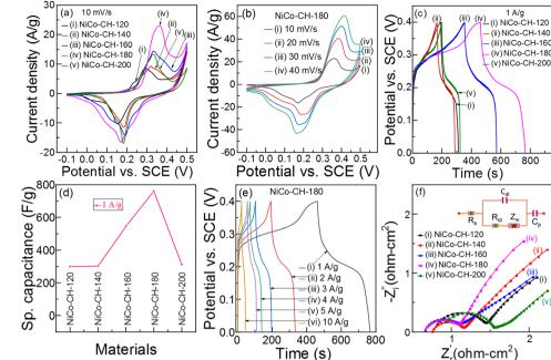
Fig. 4 (a) CV curves of NiCo-CHs synthesized at different temperatures. (b) CV curves of NiCo-CH-180 at different scan rates. (c) GCD plots at 1 A g<sup>-1</sup> and (d) specific capacitance of the NiCo-CHs synthesized at different temperatures. (e) GCD plots of NiCo-CH-180 at different current densities. (f) Nyquist plots of NiCo-CHs synthesized at different temperatures.
