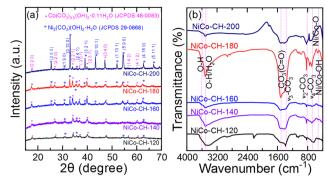
Fig. 1 (a) XRD patterns and (b) FTIR spectra of NiCo-CH prepared at different solvothermal temperatures (120, 140, 160, 180, and 200  $^{\circ}$ C) while keeping other synthesis parameters fixed, *i.e.*, 2:1 Ni: Co precursor, 15 mL EG + 20 mL water solvent, and 12 h.
