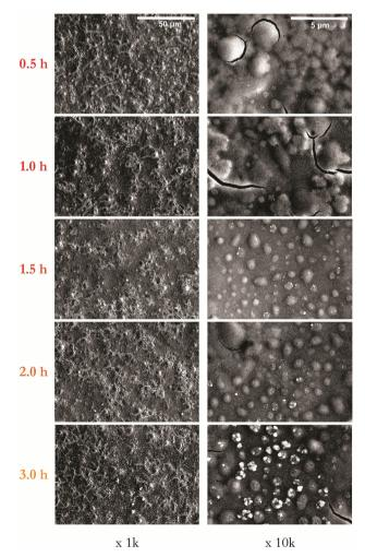
Fig. 8 Series of representative SEM images as a function of annealing at 500  $^{\circ}$ C with time from 0.5–3.0 hours shown at magnifications of 1k and 10k.
