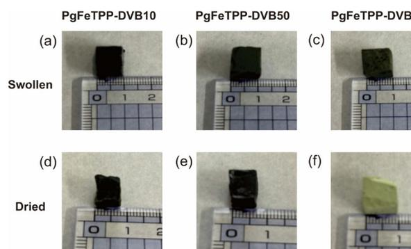
**Fig. 2** Photo images of synthesized polymers with distinct cross-linker ratios. (a), (b), and (c) represent the swollen states of **PgFeTPP-DVB10**, **PgFeTPP-DVB50**, and **PgFeTPP-DVB100** with *N,N*-dimethylformamide, respectively. (d), (e), and (f) represent the dried states of **PgFeTPP-DVB10**, **PgFeTPP-DVB50**, and **PgFeTPP-DVB100**, respectively.
