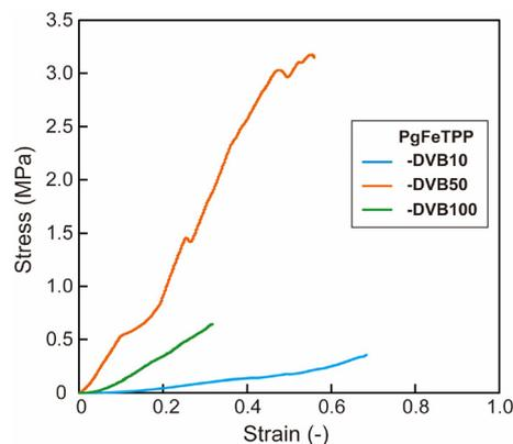
**Fig. 3** Stress–strain curves for DMF-swollen **PgFeTPP** series under uniaxial compression. Blue, orange, and green lines represent **PgFeTPP** with DVB contents of 10, 50, and 100 wt%, respectively.
