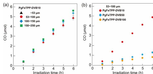
**Fig. 8** (a) Photocatalytic activity of PgFeTPP-DVB10 in each classified particle sizes. Black triangles (~53 μm), red circles (53–100 μm), blue diamonds (100–150 μm), and green squares (150–250 μm) represent the particle sizes. (b) Photocatalytic activity of PgFeTPP-DVB10 with different cross-linking ratio. DVB feed ratios to total monomer amount are 10 (red circles), 50 (blue circles), and 100 wt% (orange circles), respectively.
