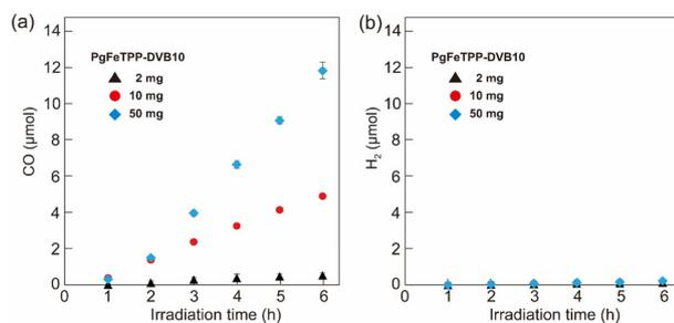
**Fig. 7** Photocatalytic activity of PgFeTPP-DVB10 at each dosage. Produced amount of carbon monoxide (a) and hydrogen (b). Black triangles (2 mg), red circles (10 mg), and blue diamonds (50 mg) represent the amount of PgFeTPP-DVB10 in the reaction solution.
