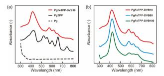
Fig. 4 Diffuse reflectance UV-vis spectra for polymer powders. (a) PgFeTPP-DVB10 (red line), PgTPP (black line), and Pg (dashed line). (b) PaFeTPP-DVB50 PaFeTPP-DVR10 (red line) PgFeTPP-DVB100 (green line).
