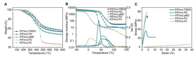
Fig. 1 Characterization of the polyimine networks: TGA (A), DMA (B) and tensile stress-strain tests (C).
