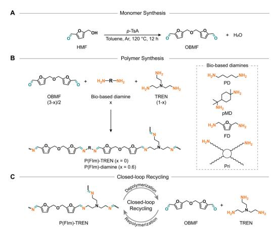
Scheme 1 Synthetic scheme for OBMF (A) and resultant furfural based polyimine networks (B). Schematic illustration of the closed-loop recycling of P(FIm)-TREN (C).
