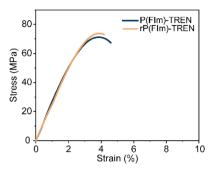
**Fig. 3** Stress-strain curves of pristine polyimine P(FIm)-TREN and chemically recycled polyimine rP(FIm)-TREN.
