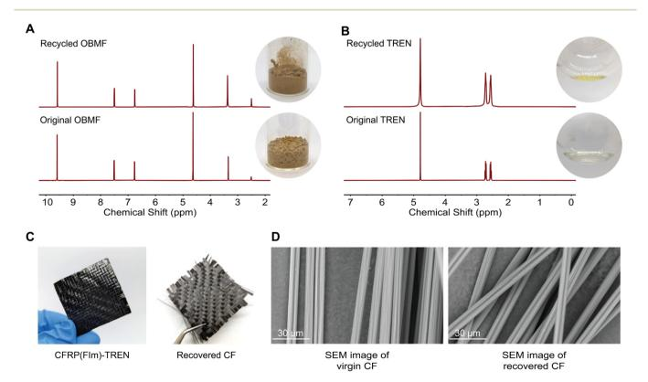
Fig. 2 Chemical recycling of P(FIm)-TREN: physical appearance and <sup>1</sup>H NMR spectra of OBMF in DMSO-d<sub>6</sub> (A) and TREN in D<sub>2</sub>O (B) after depolymerization and subsequent purification, visual appearance of CFRP(FIm-TREN) and recovered carbon fiber cloth upon depolymerization of the composite (C), SEM images of virgin and recovered carbon fibers (D). Scale bar is 30  $\mu m$ .
