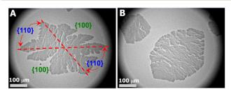
Fig. 4 OM images of a single layer LS-film for a  $X_{PtBA} \sim 0.14$  PCL/PtBA blend crystalized during an isobaric area relaxation experiment at  $\Pi$  ~ (A) 9.5 and (B) 8.5 mN m<sup>-1</sup>, respectively.
