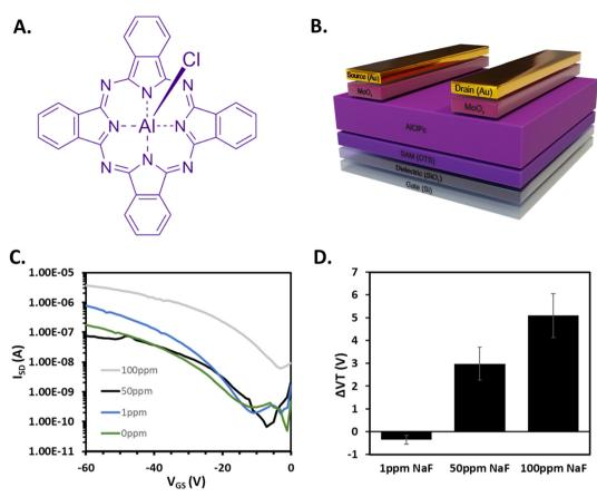
Fig. 2 Device characteristics and sensor performance. (A) Chemical structure of AlCIPc. (B) AlCIPc BGTC device structure. (C) AlCIPc OTFT transfer curves after assembly into PDMS system and after introduction of water based NaF samples at 0, 1, 50, or 100 ppm. (D) Threshold voltage change with NaF introduction to AlClPc OTFTs.
