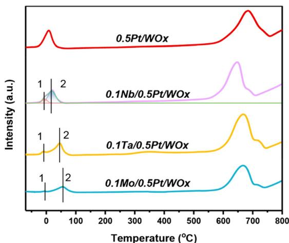
Fig. 3 H<sub>2</sub>-TPR profiles of 0.1M/0.5Pt/WO<sub>x</sub> catalysts.
