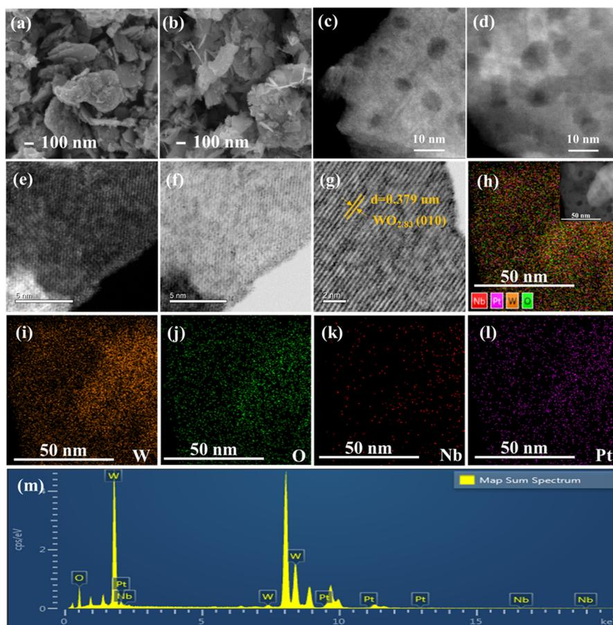
**Fig. 2** SEM and HAADF-STEM images of  $0.5\text{Pt}/\text{WO}_x$  (a and c) and  $0.1\text{Nb}/0.5\text{Pt}/\text{WO}_x$  (b and d); aberration-corrected HAADF-STEM images (e–g) and the corresponding elemental mappings (h–l) of  $0.1\text{Nb}/0.5\text{Pt}/\text{WO}_x$ , and the EDX spectrum (m).
