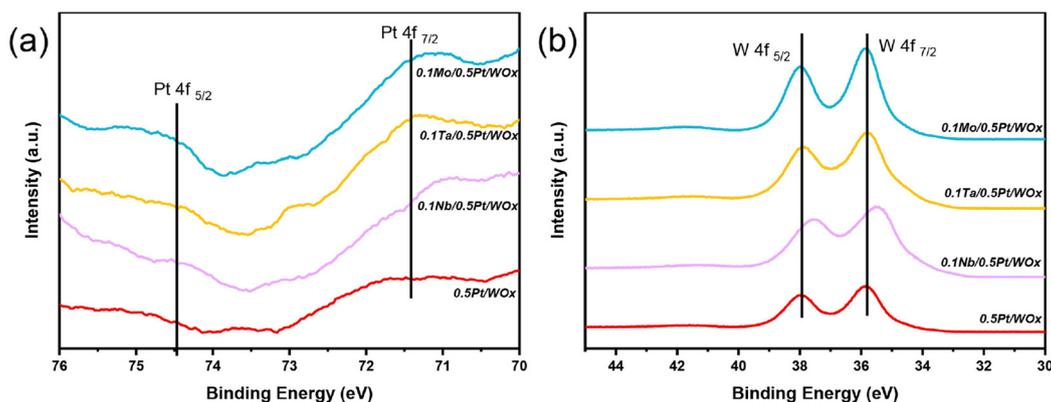
Fig. 4 XPS spectra of Pt 4f (a) and W 4f (b) for 0.1M/0.5Pt/WO<sub>x</sub> catalysts.
