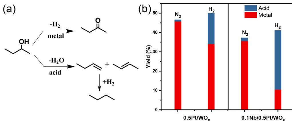
Fig. 5 (a) Reaction pathways for the dehydration/dehydrogenation of 2-butanol and (b) the performance of 2-butanol dehydration/dehydrogenation in the presence of N<sub>2</sub> or H<sub>2</sub> over 0.5Pt/WO<sub>x</sub> and 0.1Nb/0.5Pt/WO<sub>x</sub> samples.
