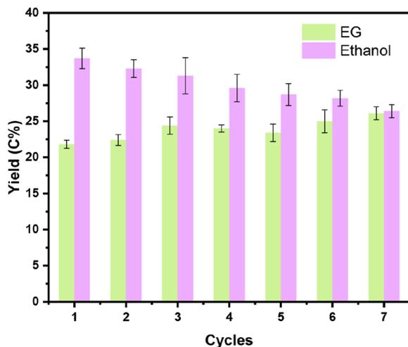
**Fig. 6** The stability tests for the catalytic conversion of cellulose over 0.1Nb/0.5Pt/WO<sub>x</sub>. Reaction conditions: 0.1 g cellulose, 0.1 g catalyst, 9.9 g H<sub>2</sub>O, 245 °C, 6.0 MPa, 2 h, 700 rpm.
