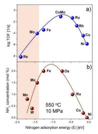
Fig. 1 The classic volcano plot for thermal-catalytic ammonia synthesis. (a) Calculated rate as a function of  $E_{\rm N}$ . (b) The NH $_3$  concentration data were taken from ref. 28. The N adsorption energies of Mn and W were taken from ref. 9.
