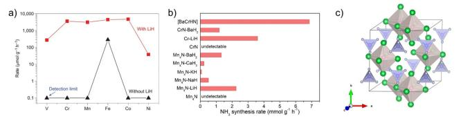
Fig. 3 (a) Impact of LiH on the catalytic activity of 3d transition metals for ammonia synthesis. Reproduced with permission from ref 14. Copyright (2017) Springer Nature. (b)  $NH_3$  production rates of a series of Cr-based and Ru-based catalysts. (c) Crystal structure of  $Ba_5CrN_4H$  (Ba, green; H, red; Cr, blue; N, gray).
