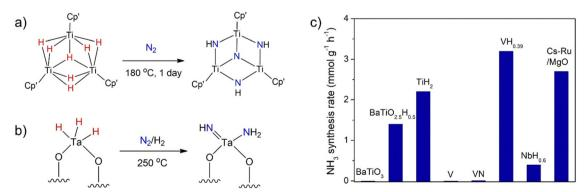
Fig. 2 (a)  $N_2$  cleavage by a soluble trititanium hydride cluster. (b)  $N_2$  activation over an isolated silica supported tantalum hydride complex. (c)  $NH_3$  synthesis rates over a series of early transition metal hydride precatalysts. Reaction conditions: 673 K, 5 MPa.
