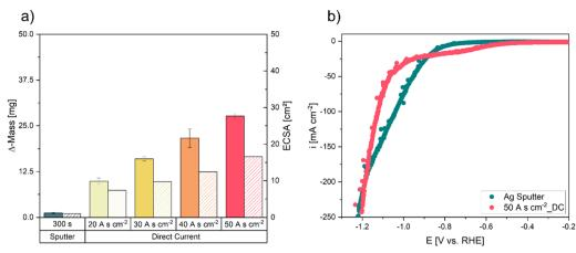
Fig. 3 Characterization of the Ag-sputtered electrode compared to the DHBT electrodes manufactured in DC mode. (a) Deposited Ag mass and ECSA values of Ag-sputtered electrode and DHBT foam electrodes with increasing charge densities during DC mode, (b) linear sweep voltammetry curves for the Ag sputter electrode and the DC-50 A s cm<sup>-2</sup> electrode to test their electrochemical performance (IR corrected potentials by applied CI method).
