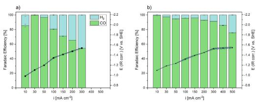
Fig. 8 Normalized faradaic efficiencies of CO and H<sub>2</sub> after galvanostatic operation at current densities up to 500 mA cm<sup>-2</sup> and the recorded WE potential after correction for the inner resistance. (a) CO<sub>2</sub>RR results of a commercial Covestro GDE and (b) CO<sub>2</sub>RR results of the Aq DHBT GDE. Each curve represents the mean of two replicate measurements with the respective standard deviations indicated by the shaded areas.
