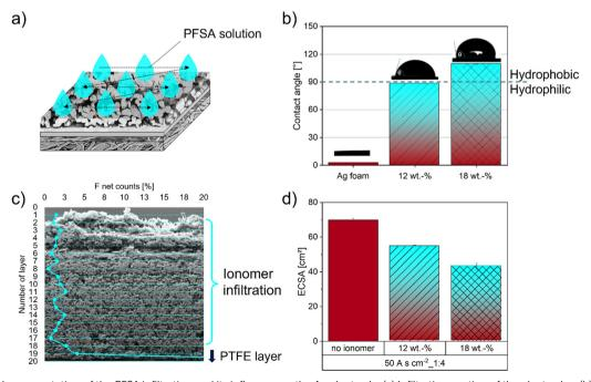
Fig. 6 Graphical representation of the PFSA infiltration and its influence on the Aq electrode. (a) Infiltration routine of the electrodes, (b) surface contact angle of the Ag foam electrodes before and after infiltration with different PFSA contents, (c) F distribution along the thickness of the GDE and (d) effect of different weight percentage of perfluorinated polymer on the ECSA of the GDE
