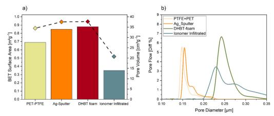
Fig. 7 Characterization of the microstructure at each processing step during GDE manufacturing. (a) Calculated BET surface area by and measured pore volume by capillary flow porometry, (b) distribution of pore diameters.
