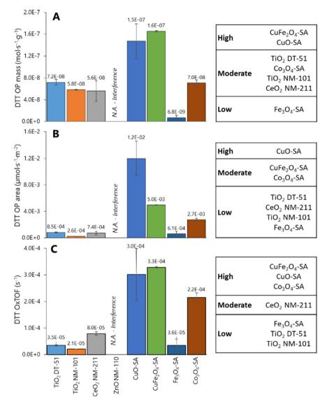
Fig. 4 Oxidative potential evaluated by DTT assay and expressed as reaction rate per mass (A), reaction rate per surface (B), and oxidative turnover frequency (reaction rate per reactive site) (C). Left: Averaged OP values (n = 3) with error bars indicating the standard deviation. Right: Statistical analysis for classification of the ENMs by OP based on Tukey's test comparison.
