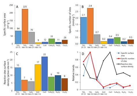
Fig. 2 Surface analysis: A) specific surface area obtained by N<sub>2</sub> adsorption isotherm, B) specific number of reactive sites obtained by methanol chemisorption, C) reactive site surface density obtained by combination of A and B, and D) comparison of the three surface descriptors (values normalized to the maximum).
