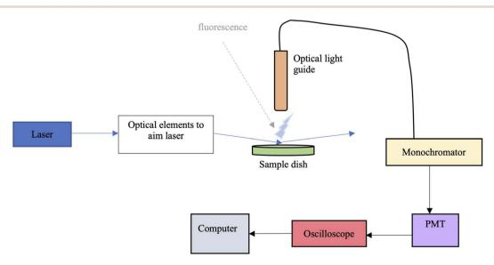
Fig. 2 Box diagram of the glancing-angle laser-induced fluorescence instrument setup.
