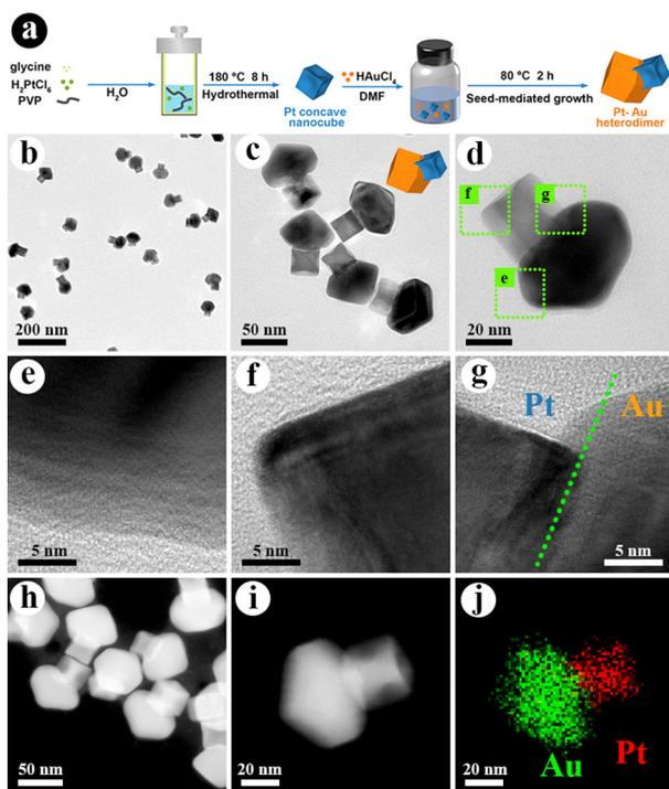
**Fig. 1** (a) Schematic diagram of the synthesis of Pt–Au heterodimers. (b)–(d) TEM images and a geometric model (inset) of the Pt–Au heterodimers at different magnifications. Corresponding HRTEM images of (e) Au, (f) Pt, and (g) the Pt–Au interface marked with green squares in panel (d). (h) Dark field STEM image of Pt–Au heterodimers. (i) Dark field STEM image of a single Pt–Au heterodimer and (j) corresponding EDS-mapping of the single Pt–Au heterodimer.
