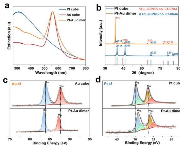
**Fig. 2** (a) UV-vis extinction spectra of Pt concave nanocubes, Au nanocubes and Pt–Au heterodimers. (b) XRD patterns recorded from Pt concave nanocubes and Pt–Au heterodimers. (c) Au 4f and (d) Pt 4f XPS spectra of Pt concave nanocubes, Au nanocubes, and Pt–Au heterodimers.
