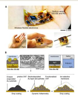
**Fig. 9** (A) Overview of a wireless all-in-one sodium sensor with a solid-state ISE (SS-ISE) and a reference electrode (RF), attached to different substrates. (B) Graphical depiction of the SS-ISE and RF, and the production steps for the SS-ISE.<sup>179</sup> Copyright 2021, Elsevier.
