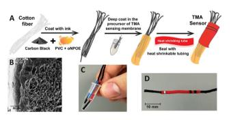
Fig. 4 (A) The process of preparing a home-made TMA sensor for vaginosis analysis. (B) A SEM cross-section image of the membrane coated TMA sensor (scale bar is 50 µm). (C and D) Photographs of the sensor depicting its portability and size. 102 Copyright 2023, MDPI.
