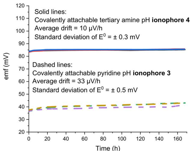
**Fig. 5** Long-term stability of PDMA membranes doped with covalently attached ionophore 4 (solid lines) or 3 (dash lines), as measured relative to an AgCl-coated Ag wire in 10.0 mM pH 7.1 phosphate buffer that contained 1.0 mM NaCl in a temperature-controlled Faraday cage at 25 °C.
