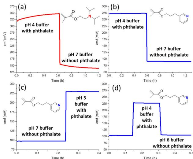
**Fig. 4** EMF of pH ISEs comprising PDMA membranes doped with (a–d) 2-(diisopropylamino)ethyl methacrylate and (b–d) 3-(pyridine-3-yl)propyl methacrylate. Buffers: pH 4, 50 mM potassium hydrogen phthalate, pH adjusted with HCl; pH 5, 50 mM potassium hydrogen phthalate/NaOH; pH 6, 50 mM phosphate buffer ( $K_2HPO_4$ ,  $KH_2PO_4$ , HCl); pH 7, 50 mM phosphate buffer ( $KH_2PO_4$ /NaOH).
